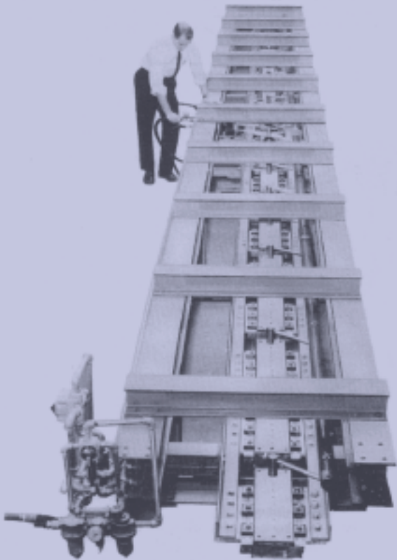
140,000 Ampere, 4.5 Volt DC, Cell Shorting Switch designed for the Chloralkali industry
